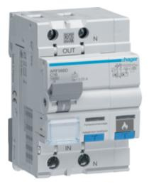
RCBO with dangerous arc detection 16A C curve 10kA Type A 30mA
