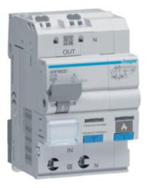
RCBO with dangerous arc detection 10A C curve 6kA Type A 30mA
