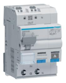
RCBO with dangerous arc detection 10A B curve 6kA Type A 30mA
