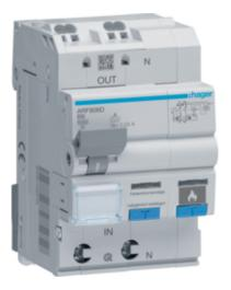
RCBO with dangerous arc detection 6A B curve 6kA Type A 30mA
