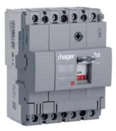
Moulded Case Circuit Breaker h3 x160 TM FIX 4P4D 50A 18kA CTC
