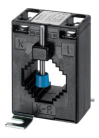
Bar/Cable-through Current Transformer BG 113 400/5A 5VA Class 1
