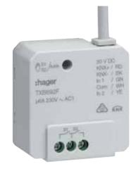
The new flush-mounted switching outputs are available as 1gang and 2gang switching outputs (in two versions). The 1gang output can be used for all types of lighting control – meaning not just switching lights on and off, but time, override, logic and scene functions too. With the 2gang output, there is the option of controlling two lighting circuits, a roller shutter/blind motor or a fan (2-stage activation).
