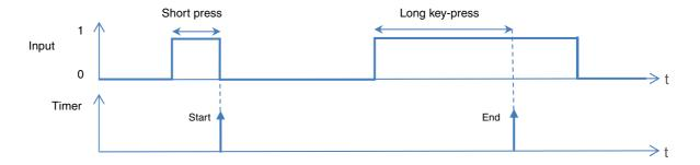
The Timer function is used to switch on a lighting circuit for a programmable period.
