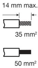
**Electrical connection for P + N for three phases only**
