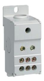
Distribution block, 160A, 1pole,  $1x 10-70^2/6x 2,5-16^2/1x$  flat copper 16x5 lateral
