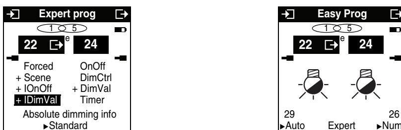
The link thus created is used to operate the output of dimmer TXA210N as a slave of the TXA215 and show the lighting level value common to the 2 outputs on the TXA215 LCD display.
