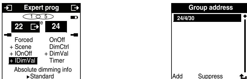
Exit and go to the right-hand part of the screen (press Num). Select the **DimVal** object of output 24, allocating the same group address to it.
