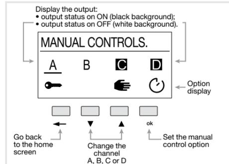
Figure 4: presentation of the manual controls screen.
