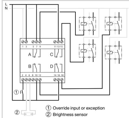
Image 3: EGN400 connection diagram (4 outputs)
