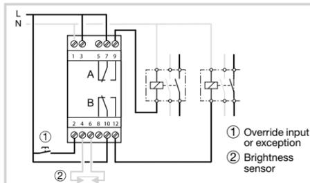
Figure 2: EGN200 connection diagram (2 outputs)
