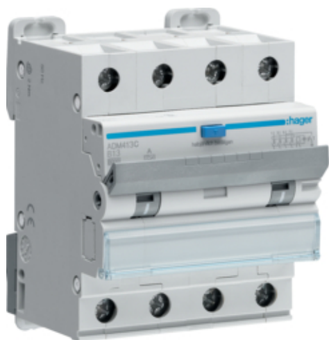
RCBO 4P 6kA B-13A 30mA A Class
