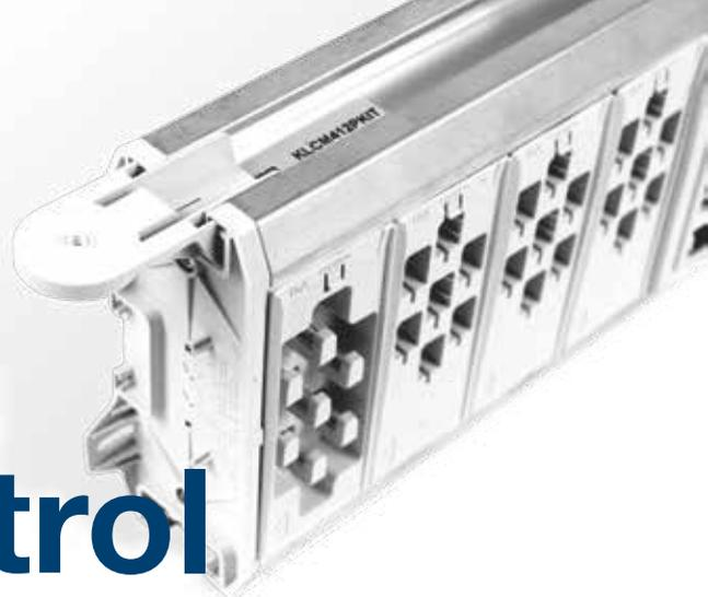
Klik LCM's (Lighting Control Module) enable the control of an area with up to 4 different control groups. Each group of outputs can control standard switched and/ or digital dimmable (DALI/ DSI) luminaires. The control module can be connected to up to 4 SELV occupancy sensors and up to 4 wall switch overrides (double retractive, centre off). Any switch or occupancy sensor can be assigned to any output.
