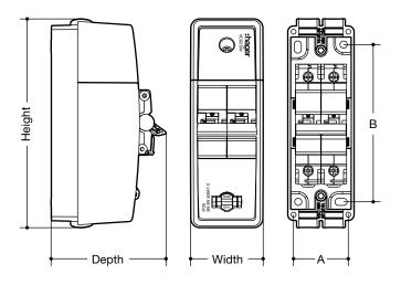
VC02SW is an Enclosed Switch Disconnector suitable for Meter Box Applications where an isolating switch between the electricity meter and consumer unit is required.
