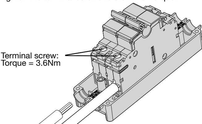
Cut/twist apart the two cable clamps and wire seal cap and trim tabs with knife/cutters as required.
