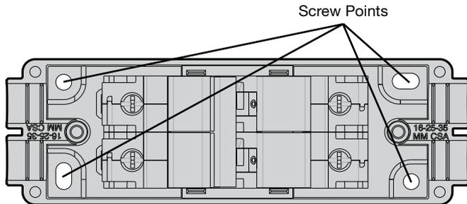
Strip/dress cables, 16/25/35mm<sup>2</sup> can be used (17mm strip length required)
