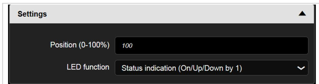
Figure 45: Entering the roller shutter position between 0 and 100 %
