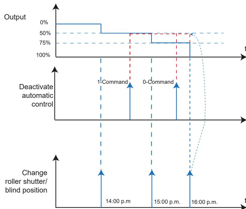
Figure 55: Signal-time diagram for Automatic control deactivation
