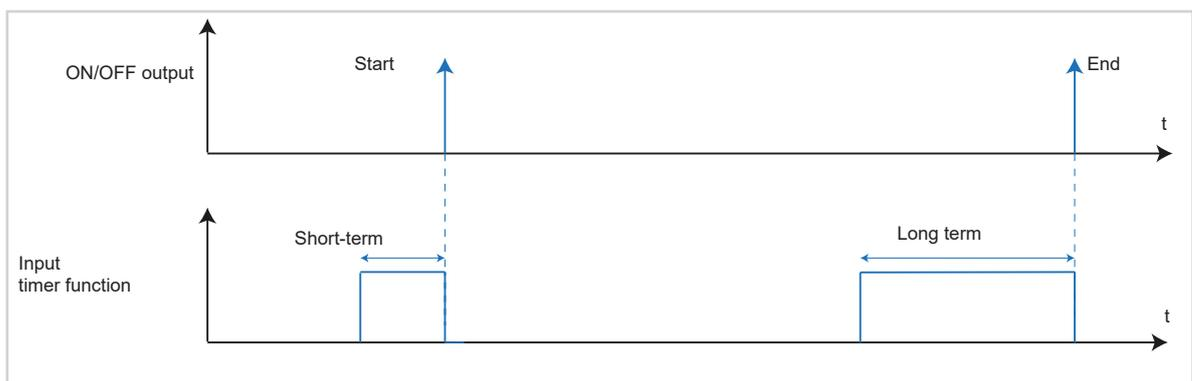
Figure 21: Signal-time diagram for timer
