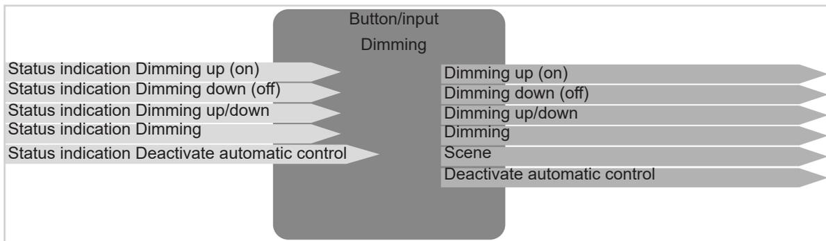
Figure 5: Input/output signals Dimming function
