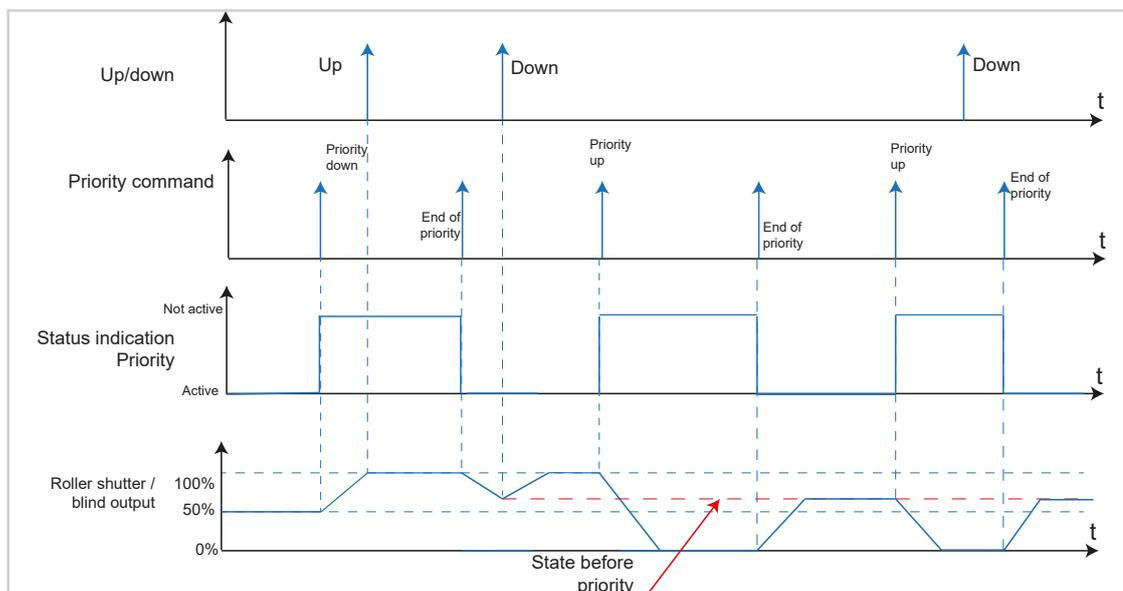
Figure 53: Signal-time diagram for **Priority roller shutter/blind**
