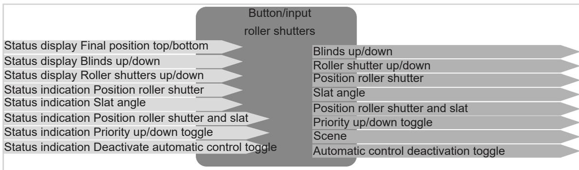
Figure 6: Input/output signals Roller shutter function
