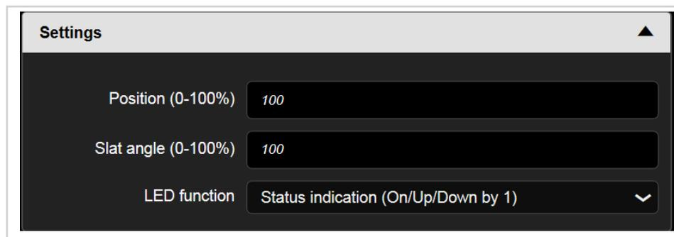
Figure 49: Entering the position/slat angle 0 - 100 %
