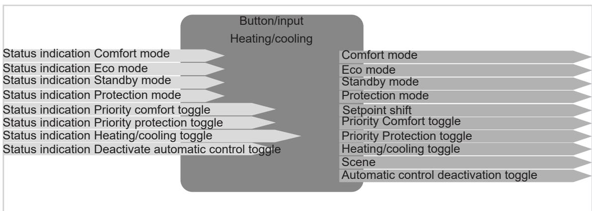
Figure 7: Input/output signals Heating/cooling function
