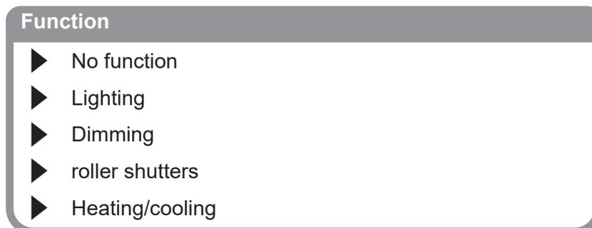
Figure 15: Function selection of the independent push-button
