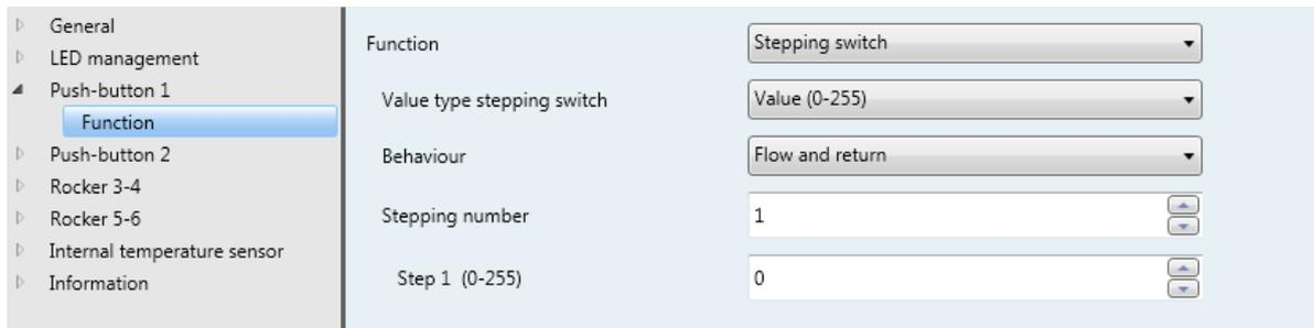
Figure 39: "Step switch" function
