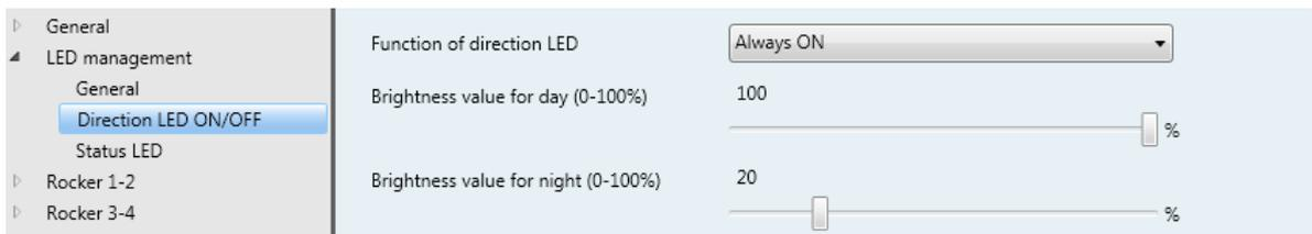
Figure 12: LED management, "Direction LED ON/OFF"
