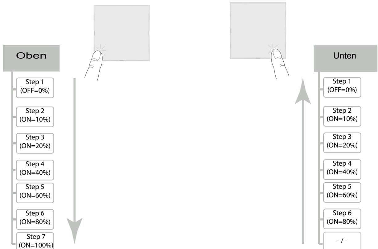
Figure 41: Stepping switch function
