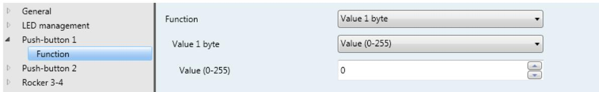
Figure 28: Function of the "Value 1 byte" independent push-button
