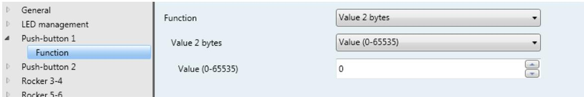
Figure 29: Function of the "Value 2 bytes" independent push-button
