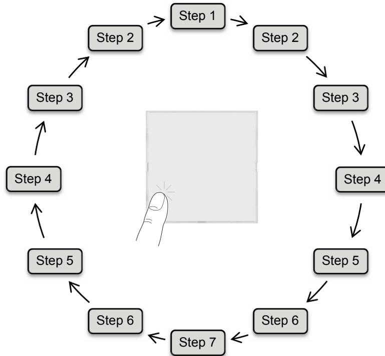
Figure 43: "Flow and return" stepping switch function
