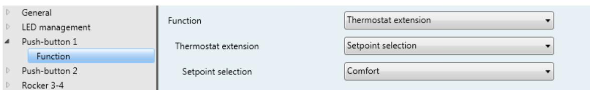
Figure 30: Function of the "Room thermostat extension unit" independent push-button
