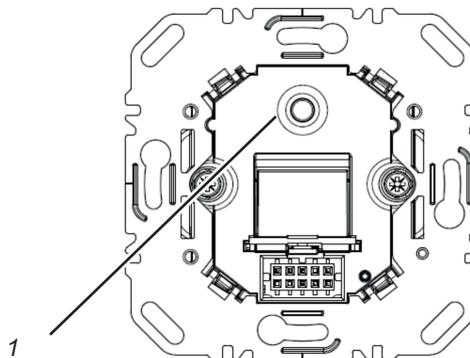
Figure 1: Bus application unit flush-mounted
