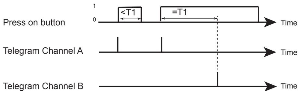
Figure 38: Channel A and Channel B operating concept
