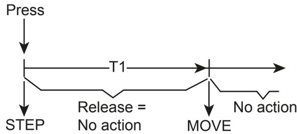
Figure 25: "Short – Long" using mode
