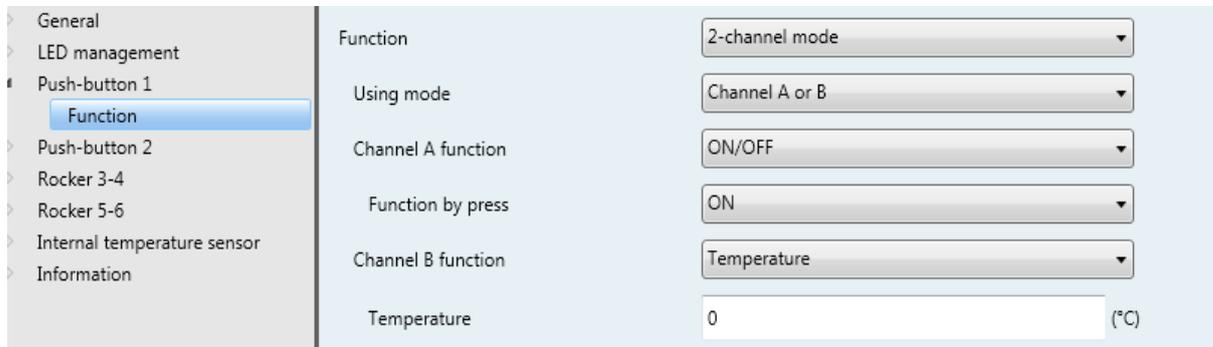
Figure 36: "2-channel mode function" parameter
