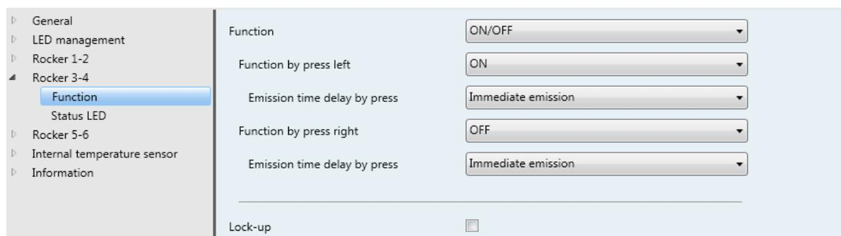
Figure 17: Function type of the rocker(s)
