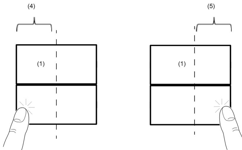
Figure 5: "2-fold rocker - S/B/K/Q" independent push-button division
